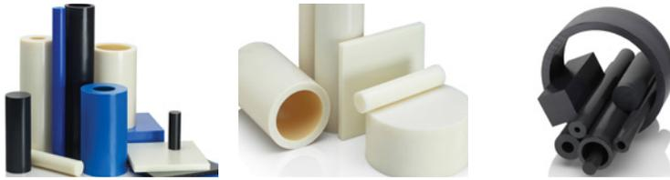
Nylon is a strong, stiff engineering plastic with outstanding bearing and wear properties. Nylon is frequently used to replace metal bearings and bushings often eliminating the need for external lubrication. Other benefits include a reduction in part weight, less operating noise, and decreased wear on mating parts.
